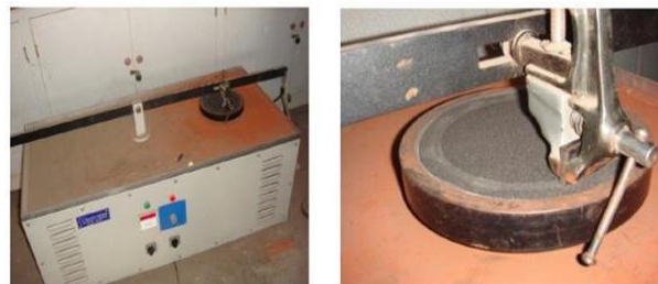
Fig 2:- pin on disc machine for abrasive wear testing
